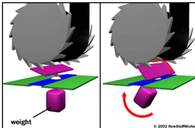
The central operating element in this mechanism is a **weighted pendulum**. When the car comes to a sudden stop, the inertia causes the pendulum to swing forward. The **pawl** on the other end of the pendulum catches hold of a toothed **ratchet gear** attached to the spool. With the pawl gripping one of its teeth, the gear can't rotate counter-clockwise, and neither can the connected spool. When the webbing loosens again after the crash, the gear rotates clockwise and the pawl disengages.
